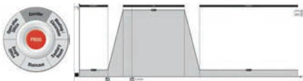
Possible DALI solution for applications in corridors: DALIeco with activated corridor function (2 changing lighting values)
